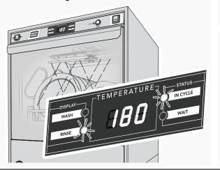
Wash cycle is extended until the final rinse temperature is a minumum of 180°F/82°C.
